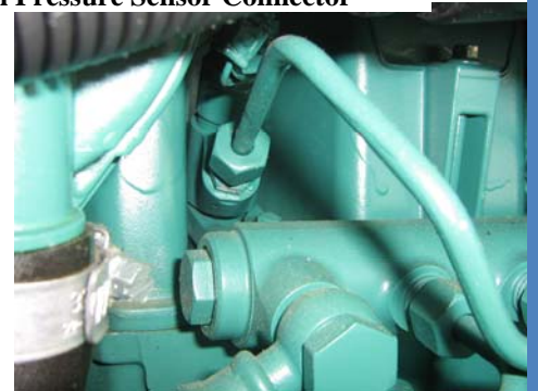
Figure 3: Fuel Relief Valve
